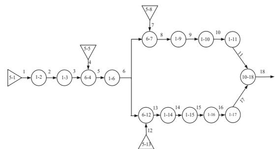
Figure 3 GO chart of hydraulic system in TAED.
