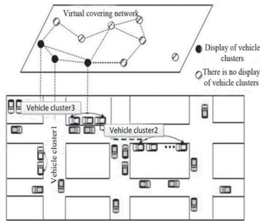
Figure 4 Virtual Overlay Network.
