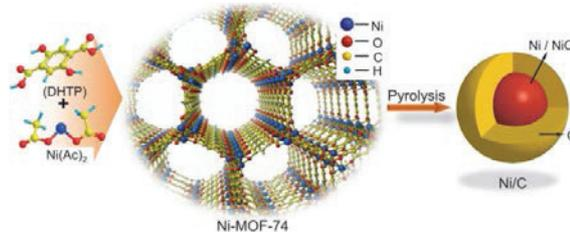
**Figure 2** The Process of Obtaining Ni/C Nano Catalyst for Battery Electrode Material.
