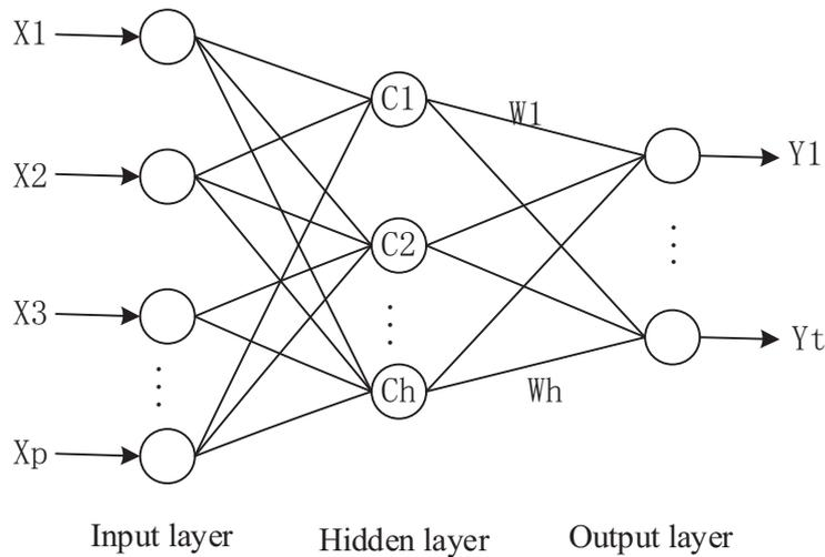
Figure 1 Three-layer feedforward NN.
