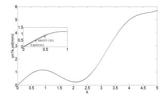
Figure 2 The output of the ordinary PD learning law and the MPD with the 20 iterations.
