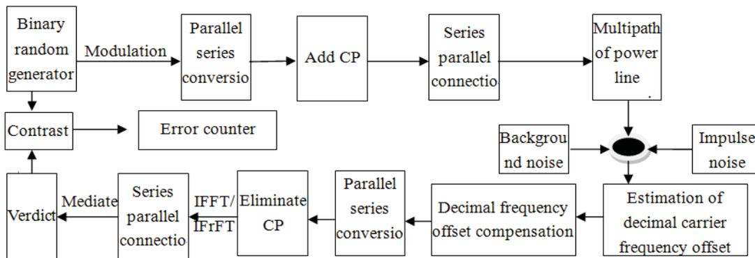
Figure 3 Simulation principle of fractional frequency offset estimation error rate.
