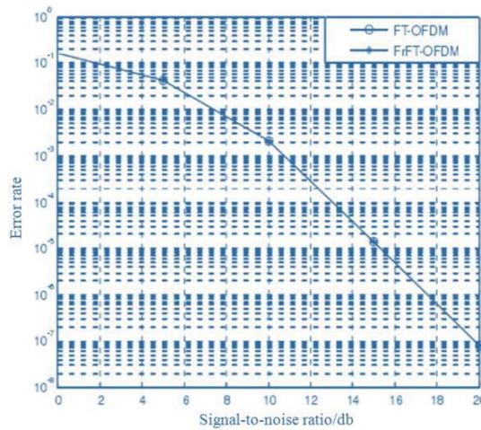
Figure 5 Bit Error Rate of Two-System Fractional Frequency Offset Estimation for AWGN Channels.
