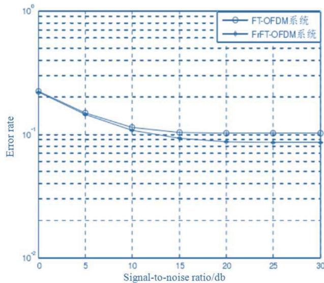
Figure 7 Bit Error Rate of Two Systems Fractional Frequency Offset Estimation for PLC Channels.
