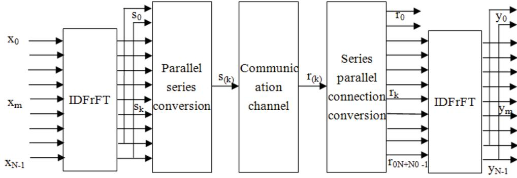
Figure 1 Orthogonal frequency division multiplexing system based on Fr FT.
