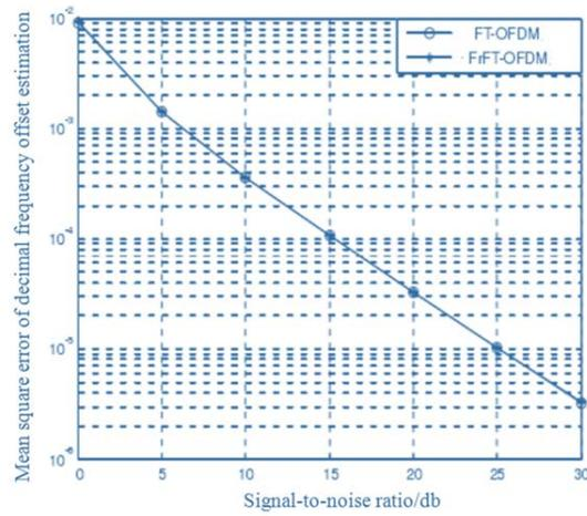
Figure 4 Mean Square Error of Two System Fractional Frequency Offset Estimation for AWGN Channel.
