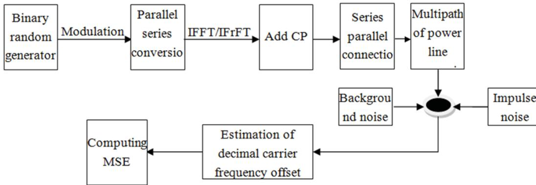
Figure 2 Simulation principle of the fractional frequency deviation estimation mean square error.
