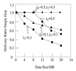
Figure 10 The Relationship Between the Rate of Transmission Success and the Amount of Data in a Single Hop.
