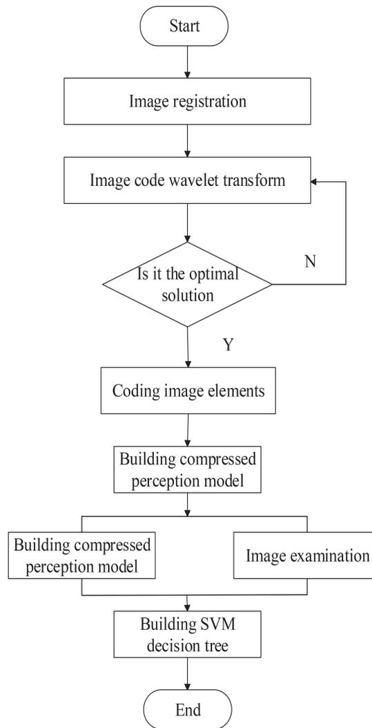
**Figure 1** Design flow of algorithm for compression perception reconstruction based on machine learning.
